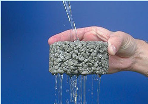
Pervious pavement at work ( www.concretedecor.net )
